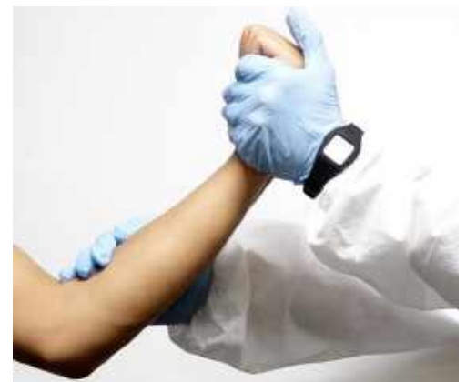
REX Kinetic Motion Detector shown correctly positioned on the testing technician demonstrates wrist and elbow flexing
