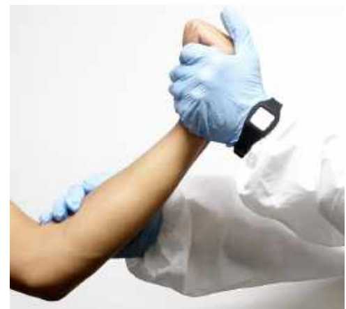
Figure 3. REX Kinetic Testing Motion Detector shown correctly positioned on the testing technician demonstrates wrist and elbow flexing.
