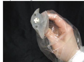
8. S - Take the elastic bands and stretch them over the draped motor, using at least two wraps. Be careful to smooth out any wrinkles from the mating flat surface of the motor as this is done, but do not touch the pins or drive plate. Ensure the wraps are above the flanges on the motor to prevent slipping.
