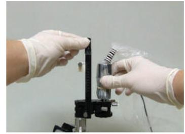
Do not attempt to manually adjust the micro-drive depth using the knobs once the motor has been mounted, as this can damage the motor.
