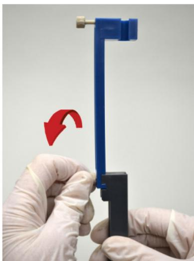
1. Secure the lead holder to the measurement fixture.
