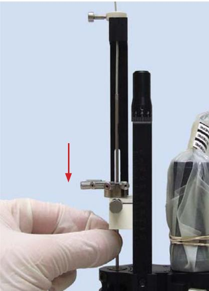
3. Insert the preset lead into the insertion tube and into the brain.
