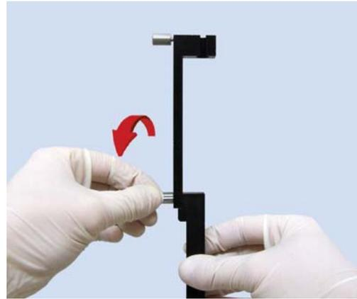
1. Secure the lead holder to the measurement fixture.
