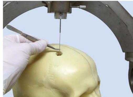
7. Secure the lead next to the skull with smooth tweezers or the selected securing device.
