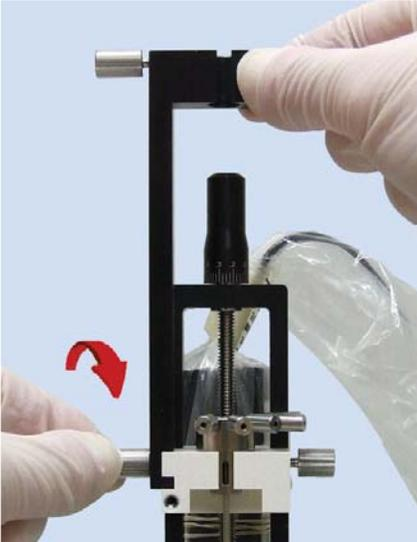
2. Secure the lead holder to the drive positioning platform.
