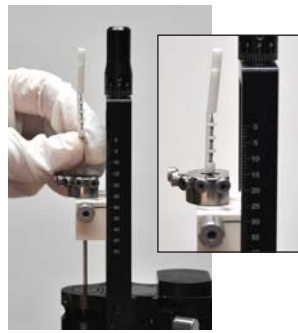
10. Insert 28cm lead in insertion tube until the lead stylet handle comes flush to the tube collar.
