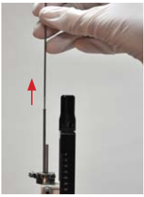
4. Remove all other microelectrode insertion tubes. (Remove lower guide spacer tubes if using a microTargeting Drive.)
