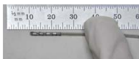
9. Select lead contact to position at target. The distance between that contact and the end of the ruler represents the distance the drive needs to be advanced.
