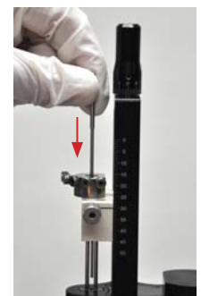
3. Insert lead insertion tube in selected track until fully seated. Holding the stylet handle down will ensure the stylet protrudes at the end of the insertion tube.
