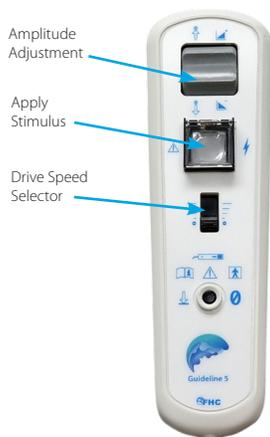
By default, stimulation will be applied only while the apply stimulus button is depressed. If the Fixed Duration check-box is checked, the button must only be momentarily pressed. The stimulation will be applied for the selected duration and stop automatically. Pressing the button again at any point during the fixed duration will cancel all stimulation immediately.
