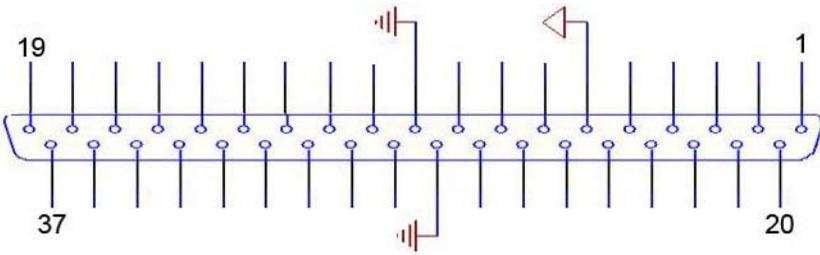
Pinout of DB37 connections on the ten-channel breakout box.
