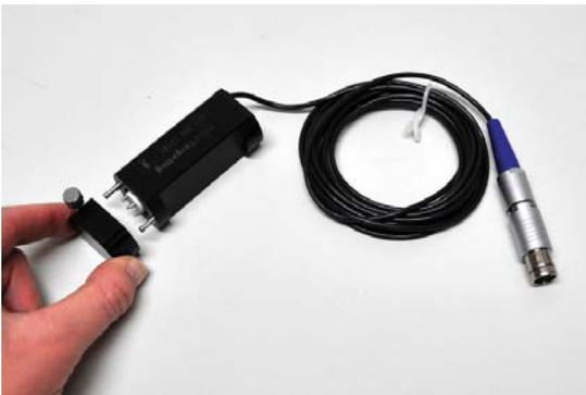
1. [STERILE] (or prior to putting on sterile gown and gloves): Remove the protective storage cap from the Motor. To remove any debris, wipe the alignment and center drive pins with an isopropyl alcohol dampened, lint free cloth or wipe. Coil the assembly's cable and place it on a flat surface so that it can be picked up with its cable in one hand.
