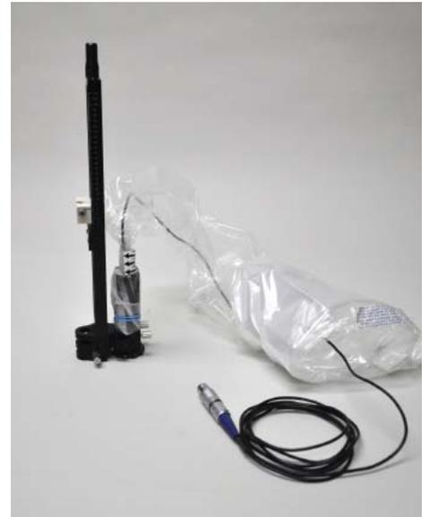
5. Tighten the Assembly locking knobs securely and test the Assembly for secure attachment and operation.
