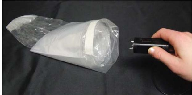
3. [STERILE] : Holding the non-sterile assembly with the pins pointing away from you, and the coiled cable in the same hand, slide it into the drape, being careful not to touch the outside of the drape.
