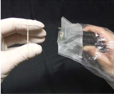
7. Take the elastic band and stretch them over the assembly, using at least two wraps. Be careful to smooth any wrinkles from the mating flat surface of the assembly as this is done. Do not touch the pins or drive plate. Ensure the wraps are above the flanges on the assembly to prevent slipping.
