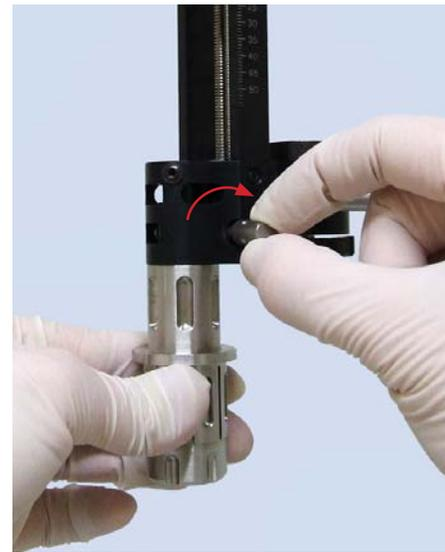
4. Secure the Stereotactic Adapter to the Drive. (See pages 15-16 for appropriate type.)
