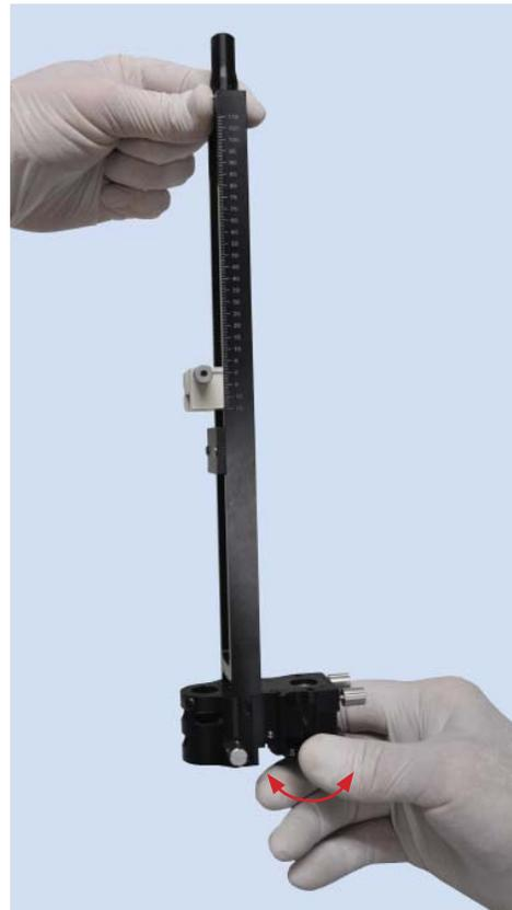
1. Check the motor transfer belt tension by grasping the upper drive adjustment screw knob ("C" on page 3) firmly. Then try to rotate the lower drive adjustment screw knob ("G" on page 3). There should be no "elasticity". If any "play" is noted, the transfer belt must be replaced. (Refer to the procedure provided with the spare parts kit 70-AC-KT-XL.)
