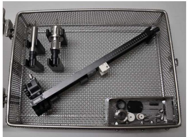
2. Tray with correct positioning of all sterilizable components.
