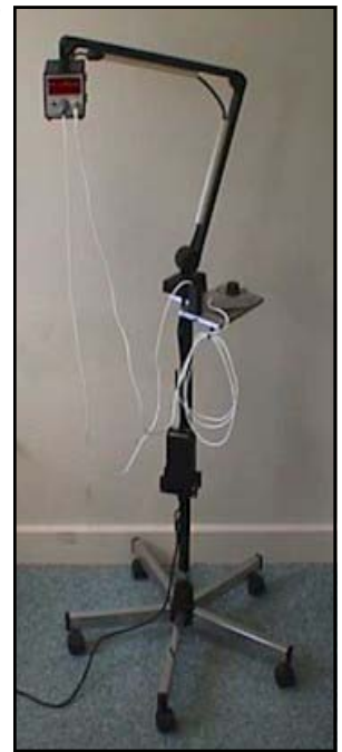
Articulating Arm and Mobile Stand shown with Power Assist Assembly, Power Assist Module, and Power Supply installed. Note coupler and Remote Control stowed on Tray for storage between procedures.
