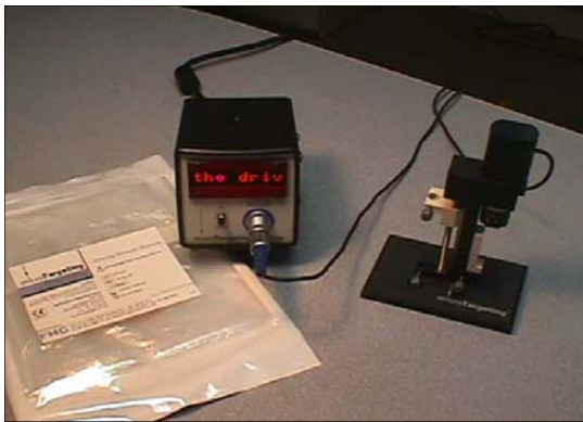
Display configuration showing Display Assembly mounted on microTargeting™ Drive (Adapter Kit installed), Sterile Sleeve not installed.
