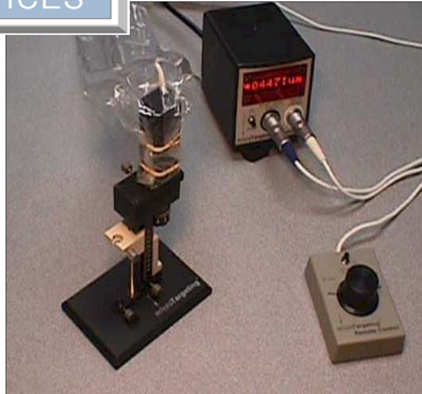
Power Assist Assembly with Sterile Drape Sleeve shown assembled on the microTargeting™ Drive and Mounting Stand, connected to Power Assist/Display Module with Remote Control.
